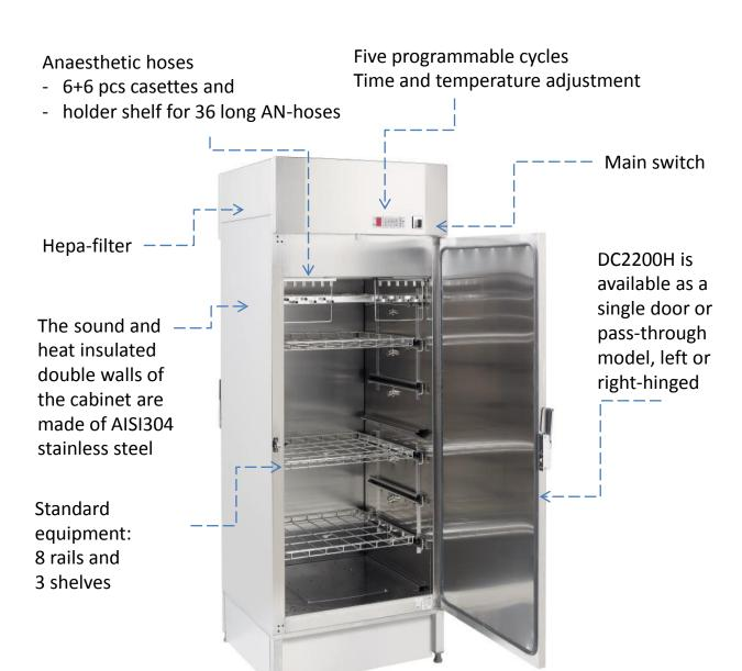
DC2200H Drying cabinet is designed especially for drying surgical instruments, anaesthetic hoses & equipment, as well as other re-usable items used in patient health care.
